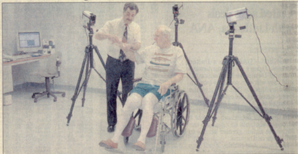
Senior Research Scientist Alexander Aruin, left, explains to Frank Bauman how the new Motion Analysis system works. The cameras pick up movement of the sensors and feed the information to a computer for analysis.
