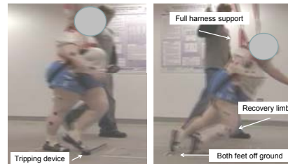
Figure 2. (left) In Study 2, subjects walked while wearing a full body safety harness. A pneumatic obstacle was triggered to rise from the laboratory floor and obstruct the motion of the foot of the swing limb (right). Four of five obese fallers, became fully supported by the harness before the recovery limb was able to complete the step (right). Kinematics at recovery step completion could not be calculated for these fallers. All normal weight subjects were able to complete the recovery step.
