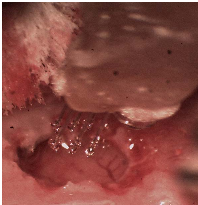
Fig.3 A six channel microwire recording electrode made of 50um tungsten wires encased in 140um polyimide tubes. Each wire is spaced 400um center to center apart. The guide tube for the stroke induction can be observed on the right side of the array.
