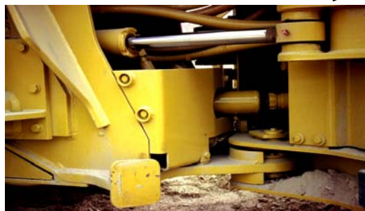
Enlarged view: steering hinge joint and hydraulic cylinder (a pair)
