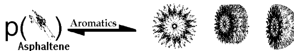
Fig. 4. Micellization (self-association) of asphaltene due to increase in aromaticity (polarity) of its medium.
