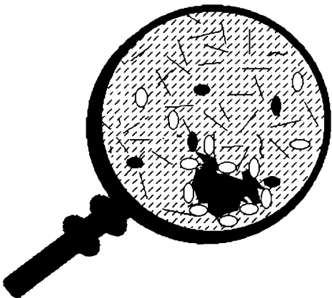
Fig. 4. Steric colloidal phenomenon due to increase in concentration of paraffinic hydrocarbons in crude oil.
