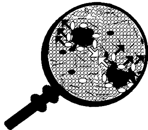
Fig. 5. Migration of peptizing molecules (shown by solid arrows ) from the surface of heavy organic particles due to the change in their chemical-potential balance between the bulk oil phase and the surface phase. This causes the potential for aggregation ( open arrows ) of heavy organic particles due to development of free active sites on their surfaces, and their eventual flocculation as shown below.
